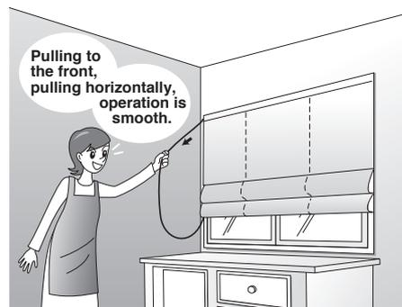
Freel's heart cam stopper makes it possible to pull the cord at any angle for stop and release operation.
