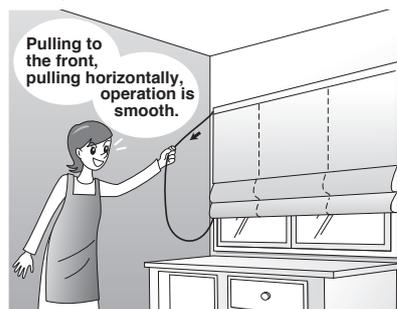
Creaty Cord's heart cam stopper makes it possible to pull the cord at any angle for stop and release operation.
