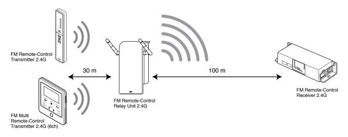
• Using FM Multi Remote-Control Transmitter and FM Remote-Control Relay Unit, it can operate TOSO motorized products without any wiring.
