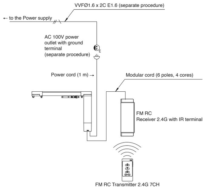
FM Remote-Control Receiver/Transmitter 2.4G Parts
