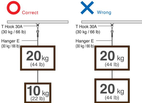
**CASE 02** If using more than one hanger to hang an article, hang with no more than two hangers and do not exceed a load of 30 kg (66 lb). (If the interval between hangers is more than 1 m/39", it should be performed in the same way.)
