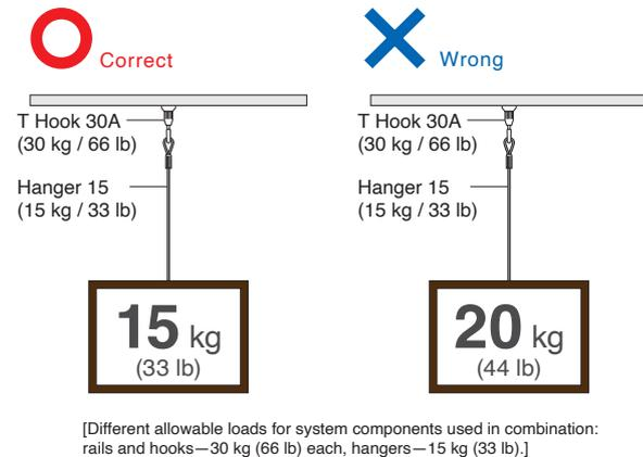
**CASE 04** If installing Rail T-1 on a wall attachment, the allowable load is 20 kg (44 lb).
