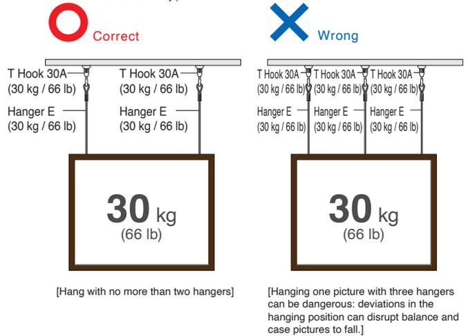
**CASE 03** If system components (rail, hook, etc.) with different allowable loads are used in combination, the smallest allowable load applies.
