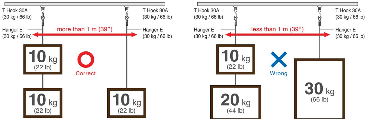
\*Although the shortest available interval between hangers is 1 m (39"), we recommend allowing a sufficient interval (more than 1 m/39") when hanging plural picture frames to prevent picture frames from colliding with each other during earthquakes, etc.
