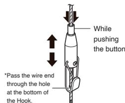
Slide the hanger hook up and down while depressing the hanger hook button. Before hanging the picture, confirm that the hook is locked and won't move down.
