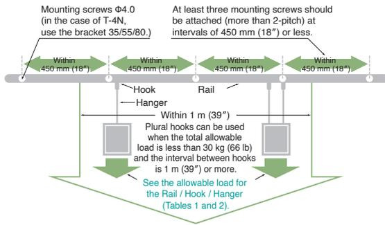
\*Plural hooks can be hung when the total allowable load is within 30 kg (66 lb) and the interval between hooks is 1 m (39") or more.
