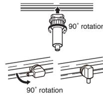
When using a one-touch hook, insert the straight hanger from the insertion hole of the hook as shown in the illustration until the tip of the wire hits the top of the hook. To unplug the wire, push the button and pull the wire out.
