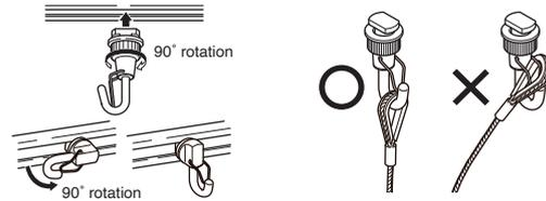
When using a standard-type hook, catch the loop part of the hanger on the hook as shown in the illustration. The carabiner-fitted type safeguards against falling articles when earthquakes strike. This is a recommended feature for public buildings or any other space visited by large numbers of people.
