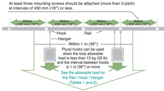
\*Plural hooks can be hung when the total allowable load is within 15 kg (33 lb) and the interval between hooks is 1 m (39") or more.
