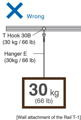
**CASE 05** When using plural hooks and hangers: if the total allowable load is within 30 kg (66 lb) and the interval between hangers is 1 m (39") or more.
