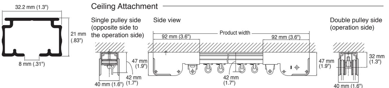
\*Allowable curtain weight for single side opening is 30 kg/66 lb (an extra 30 kg/66 lb for double side opening).
