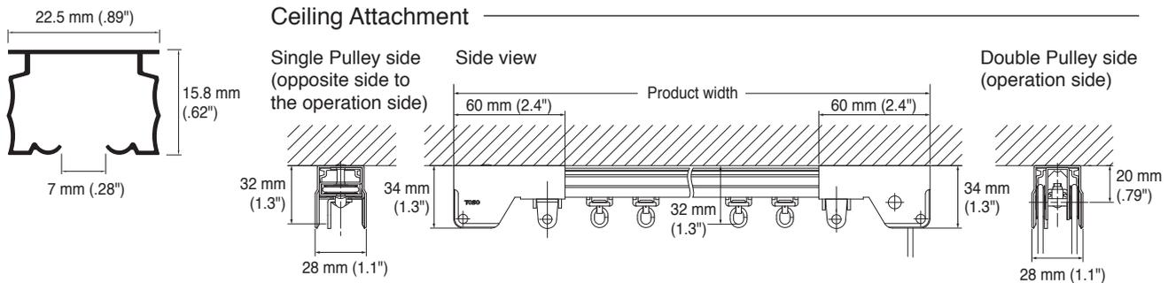
\*Allowable curtain weight for single side opening is 10 kg/22 lb (an extra 10 kg/22 lb for double side opening).
