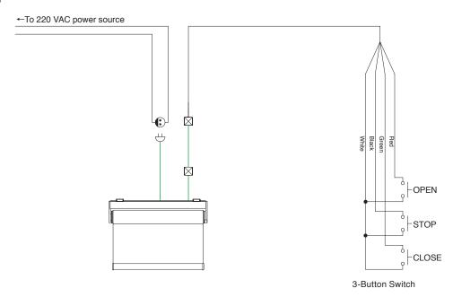
Explanatory notes: — Power supply, — Low voltage control line, — Main body attachment or TOSO standard
