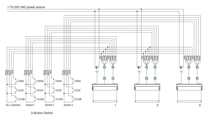
Explanatory notes: — Power supply, — Low voltage control line, — Main body attachment or TOSO standard
