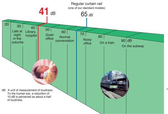
\*Noise level measured at a distance of 50 cm (20") from a 2 m (79") rail with rollers or sliders tilted at an angle of 15 degrees.
