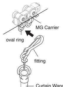
Hook the fittings of the Curtain Wand to the oval ring of the MG Carrier.
