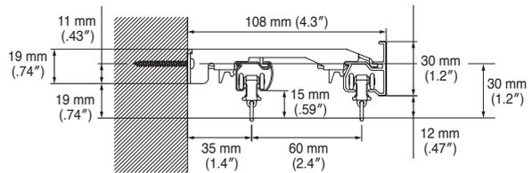
\* For attach it to the ceiling, keep the ceiling and the top of the bracket at least 10 mm apart.
