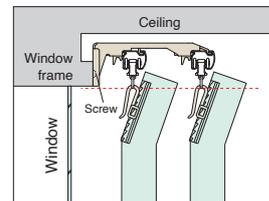
This bracket hangs the curtain higher than regular brackets. Because the top of the curtain is positioned higher than usual, very little light filters into the room. A screw hole is provided on the bottom of the bracket to enable easy installation on a window frame close to the ceiling.
