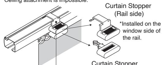
Adjust to the desired location by placing a finger here and pushing.
