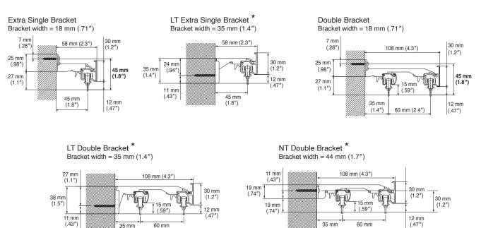
\* For attach it to the ceiling, keep the ceiling and the top of the bracket at least 10 mm apart.
