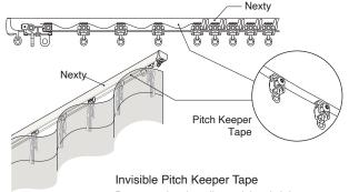
By connecting the roller and the pitch keeper tape, it can create a beautiful curtain wave. The pitch keeper tape fits inside the track for a clean look.
