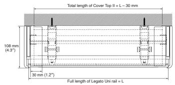
Cut dimensions when using Cover Top II Joint = (L  $\div$  2) – 20 mm
