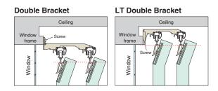
This bracket hangs the curtain higher than regular brackets. Because the top of the curtain is positioned higher than usual, very little light filters into the room.
