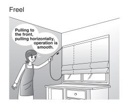
Freel's heart cam stopper makes it possible to pull the cord at any angle for stop and release operation.
