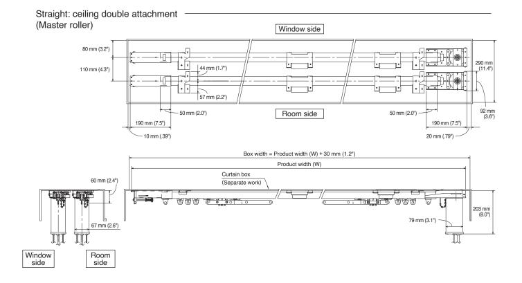
Straight: ceiling double attachment (Room side: Rail overlap, Window side: Master roller)
