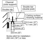
Joist foundation / Built-in rail for ceiling (Both collars)
