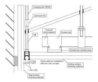
Mortar wall / Built-in rail for ceiling
