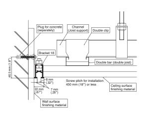
Light gauge steel wall / Built-in rail for ceiling
