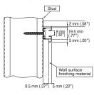
Concrete wall / Built-in rail for ceiling
