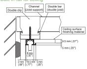
Built-in rail for ceiling (Using reinforcement plate)
