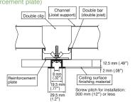
C shape steel + Hanger bolt / Built-in rail for ceiling
