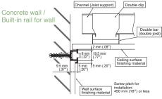
Concrete wall / Built-in rail for ceiling
