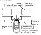
C shape steel + Hanger bolt / Built-in rail for ceiling
