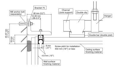
Mortar wall / Built-in rail for ceiling
