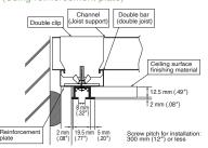
C shape steel + Hanger bolt / Built-in rail for ceiling
