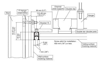
Light gauge steel wall / Built-in rail for ceiling
