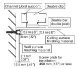
Joist foundation / Built-in rail for ceiling (One side collar)
