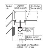
Concrete wall / Add-on rail for ceiling
