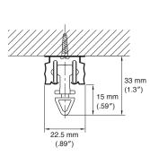
Ceiling Single Bracket Bracket width = 18 mm (.71") 57 mm (2.2") 45 mm (1.8") 15 mm (1.4") 35 mm (1.4")
