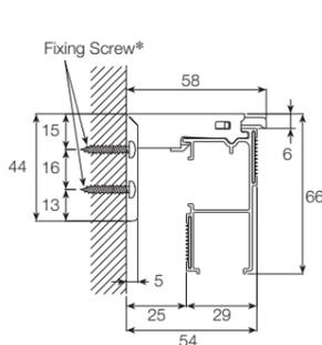
\* Universal Bracket is standard part for Front and Ceiling Attachment.
